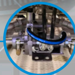
Sicherheitsventil an jeder Lenkachse Safety valve on each steering axle
